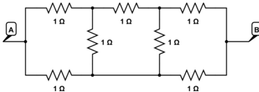
Find the equivalent resistance between points A and B. \_\_\_\_\_
