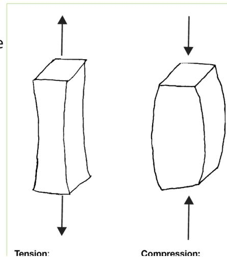
When stress is applied to the structure at the loading point, that stress is distributed throughout the structure, and each individual piece within the structure is put into two different conditions: it is either under a compression force, or a tensile (tension) force. There are more forces which can act on a piece within a structure but those two are the most relevant.
