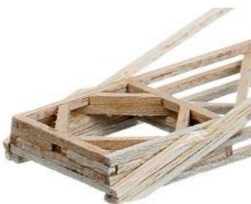
The next thing to think about is the place where the tension and compression piece meet, which is also where we will be placing the loading block. This is the most critical of all the joints, and it needs to be the most sound out of all of them. A good idea is to add more surface area so the joint is as sound as possible, there are many ways to do that, one is shown in the picture to the left.
