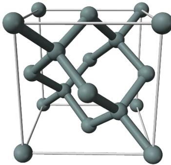
a) Observe the unit cell given above. How many atoms are in one unit cell of a silicon?
