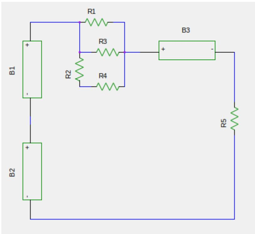
All of the resistors have a resistance of  $1.000\text{ k}\Omega$ .
