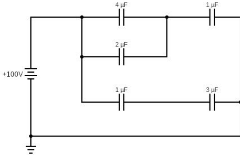
9. What is the total (equivalent) capacitance of the circuit across the battery (3 points)?
