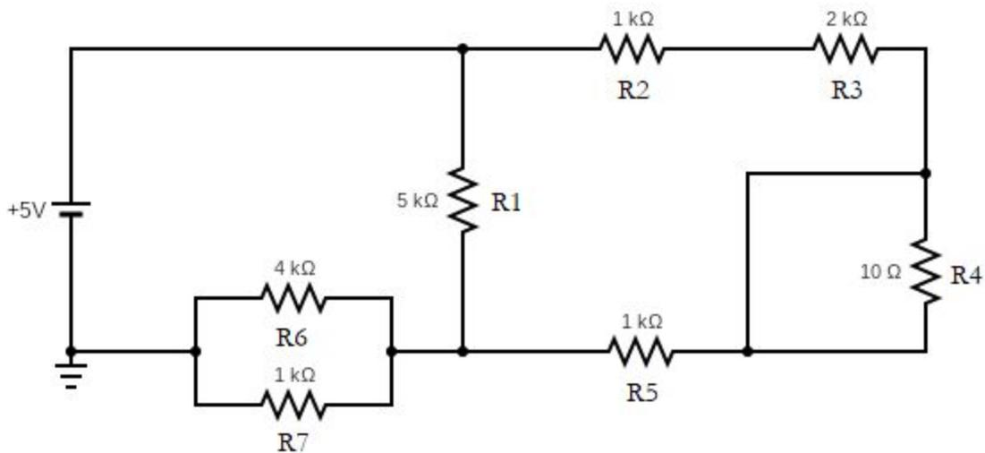
2. Calculate the voltage across each resistor. (0.5 point each)
