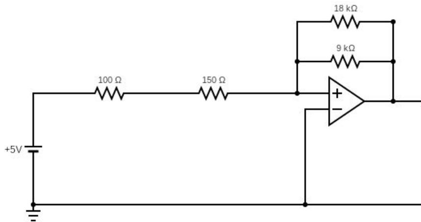
5. Assuming an ideal op-amp, find the voltage gain (output/input) of the network. (4 points)
