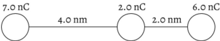
$$k\left(\frac{qq_1}{r_1^2}\right) + k\left(\frac{qq_2}{r_2^2}\right) = F_{net} \text{ (Coulomb's Law, force on center by right plus force on center by left is}$$
