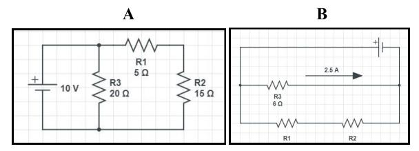
1. Determine the current running through all 3 resistors in diagram A. (4 points) (TB2)
