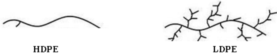
Figure 1: Structure of HDPE and LDPE
