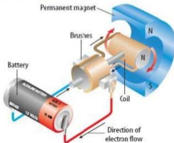
**A** A battery causes an electric current to flow through the coil of the electromagnet.
