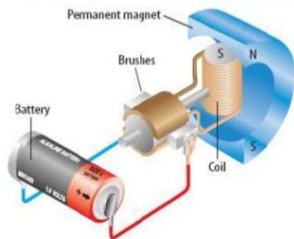
**B** Unlike poles of the two magnets attract each other, and the like poles repel. This causes the coil to rotate until the opposite poles are next to each other.
