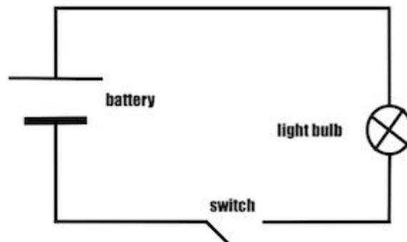
A **resistive circuit** is a circuit containing only resistors and ideal current and voltage sources. Analysis of resistive circuits is less complicated than analysis of circuits containing capacitors and inductors. If the sources are constant (DC) sources, the result is a DC circuit. For a random resistor network, the effective resistance and current distribution properties of the network can also be modeled in terms of graph measures and geometrical properties of network.
