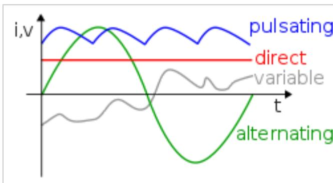
Direct Current (red line). The vertical axis shows current or voltage and the horizontal 't' axis measures time and shows the zero value.
