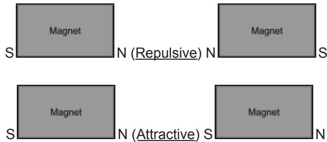
**Magnetic Pole**- Each magnet has two ends (N and S) where the magnetic effect is strongest.
