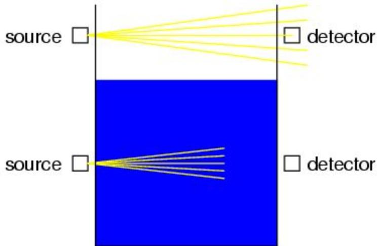
Both source and detector are outside of the vessel, with no intrusion at all except the radiation flux itself. The radioactive sources used are fairly weak and pose no immediate health threat to operations or maintenance personnel.
