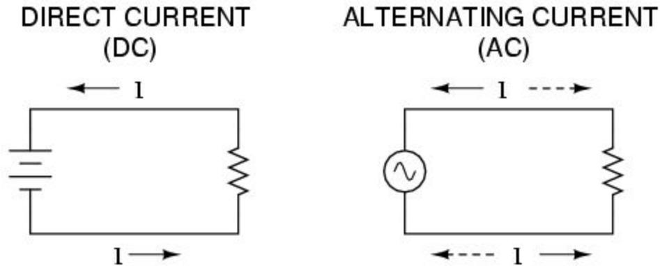
**DC** - Direct current (DC) is the unidirectional flow of electric charge. A battery is a good example of a DC power supply. Direct current may flow in a conductor such as a wire, but can also flow through semiconductors, insulators, or even through a vacuum as in electron or ion beams. The electric current flows in a constant direction, distinguishing it from alternating current (AC).
