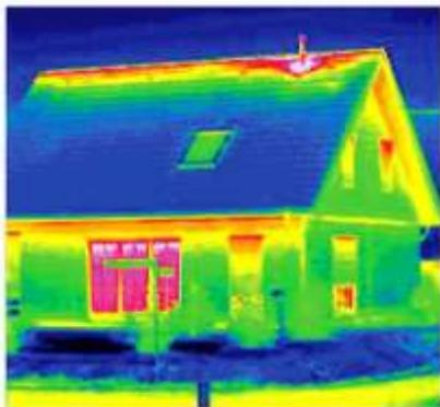
The area's in this picture that are white or Red indicate the area's where heat loss is the greatest. The closer the color is to red, the more heat that is lost from the home. The larger the area of the high temperature, the larger the amount of heat loss.
