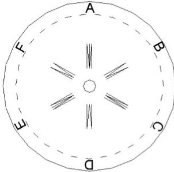
Next, fill the container provided approximately  $\frac{3}{4}$  full with the 70% alcohol located at the communal liquids table. Using the blank filter disk, roll it into a tube and insert it into the center hole to form a wick. Now place the lower end of the wick in the eluting solution, allowing the disk to lay flat across the rim of the container.
